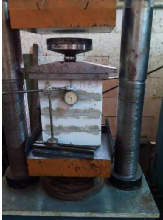
Picture 3 – Picture test samples in the press
