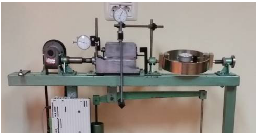
Picture 1 – The direct shear apparatus
