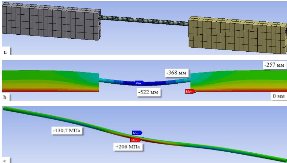
**Picture 4 – Determination of the stresses and deflection in the pipeline in the karst cavity area (cavity length  $l = 32$  m):**
