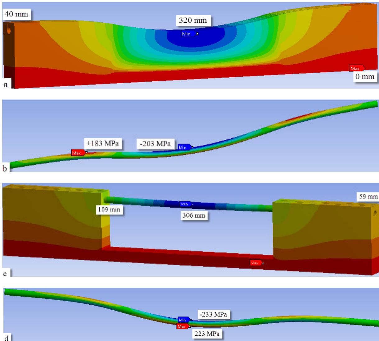
**Picture 7 – Results of the hypothesis testing that pipeline deformation equivalent to soil deformations:**
