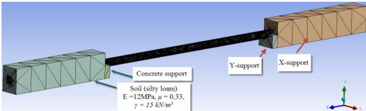
**Picture 2 – Oil pipeline above ground crossing of the ravine design scheme**
