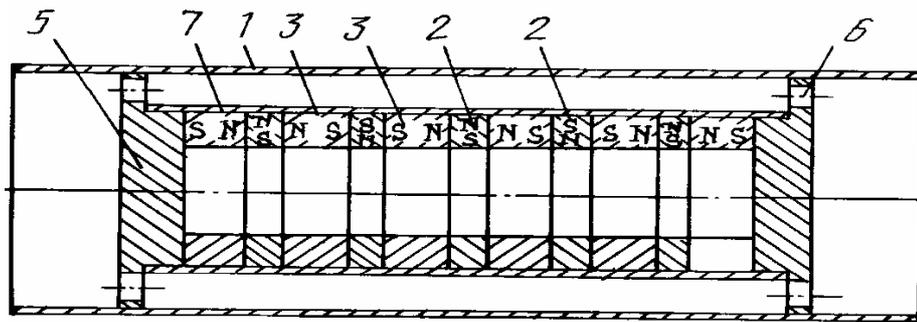
**Picture 2 – Schematic diagram of a magnetic anti-paraffin unit (MAU-1) with mutually perpendicular directions of magnetization of the magnet ring:**
