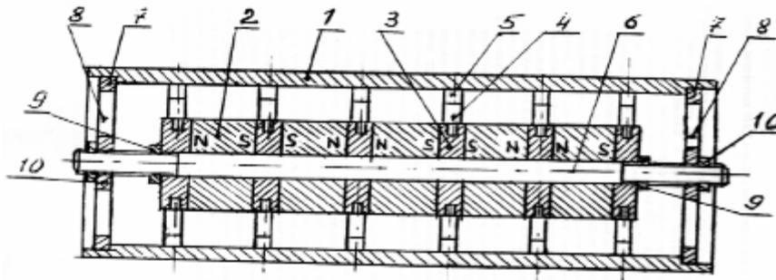
**Picture 1 – Block diagram anti-paraffin magnetic unit (MAU):**
