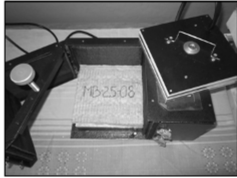
Picture 4 – Determination of thermal conductivity: a) the measuring ITC-1 device; b) process of sample installation
