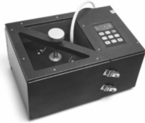
Picture 4 – Determination of thermal conductivity: a) the measuring ITC-1 device; b) process of sample installation
