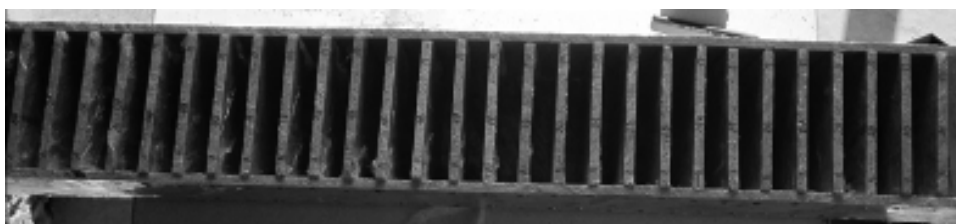
Picture 2 – Formwork for making PSC-plates experimental samples
