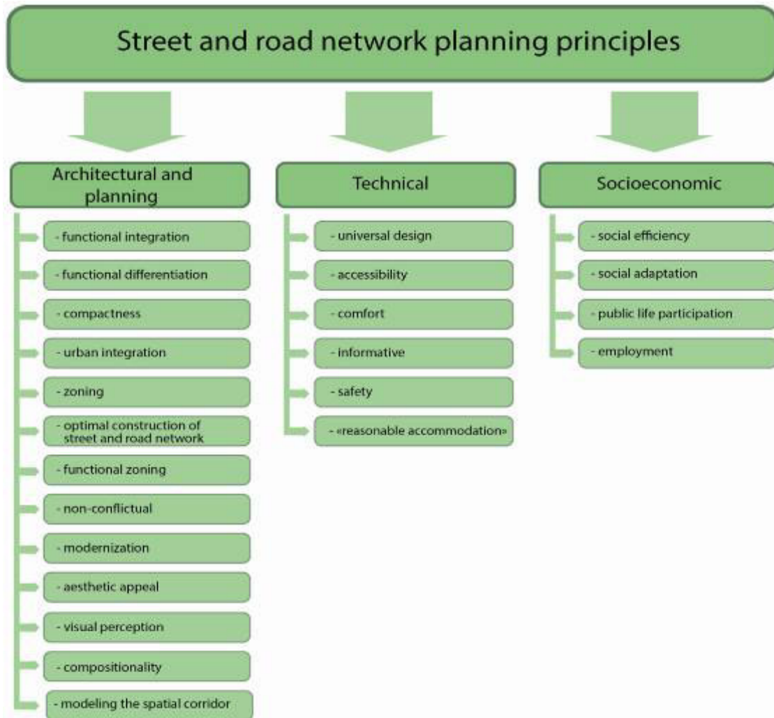
Figure 1 – Groups of street and road network design principles for needs of people with limited mobility
