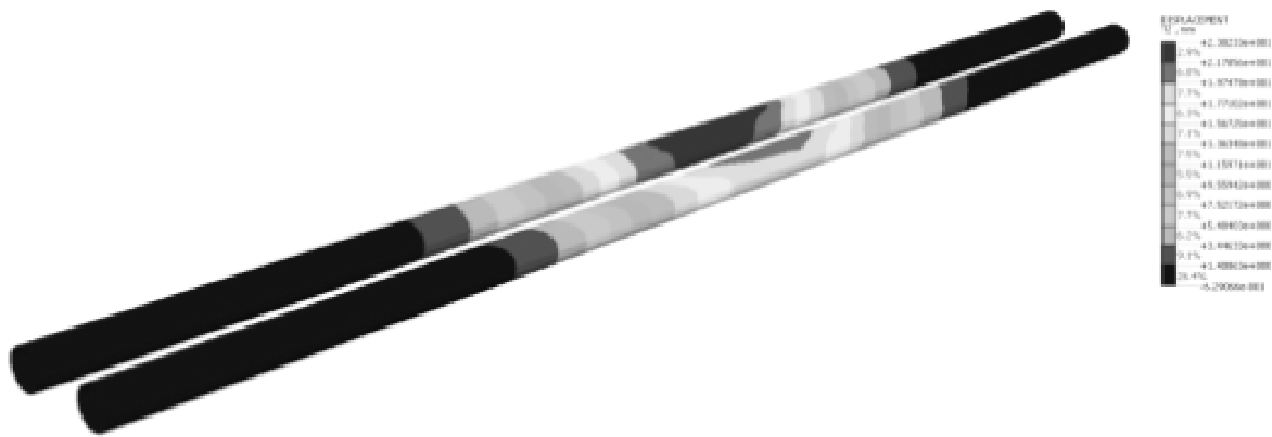
Figure 7 – Deformations arising in the lining of tunnels, without performing protective measures
