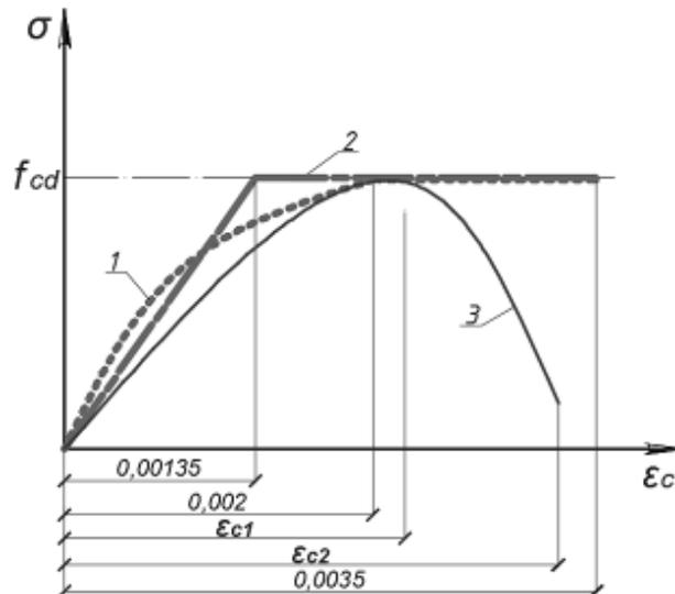
**Figure 5 – Diagrams of concrete deformation during compression:**
