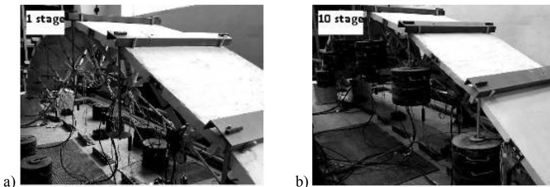
**Figure 10 – Prototype of steel and concrete composite cable space frame prototype testing**
