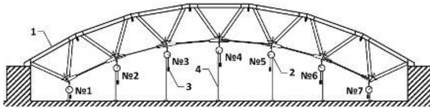
**Figure 6 – Placement of instruments for measuring displacements:**
