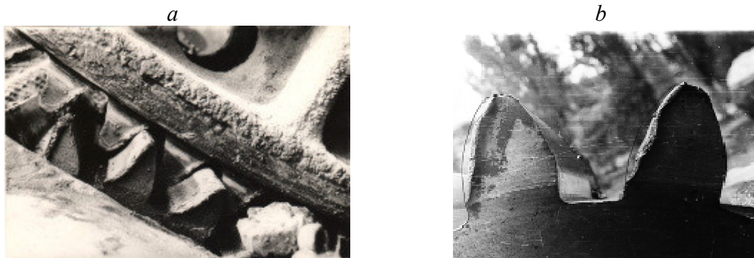
Figure 2 – Profiles of the open gear wheels gear during their long-term operation: a – the pinion and the crown wheel; b – pinion
