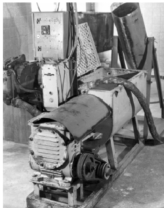
Figure 3 – Experimental installation for grout pumps study
