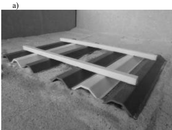
Figure 4 – Models of the folded foundation structures in assembled state: a) the first model; b) the second model
