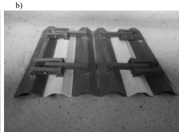
Figure 4 – Models of the folded foundation structures in assembled state: a) the first model; b) the second model
