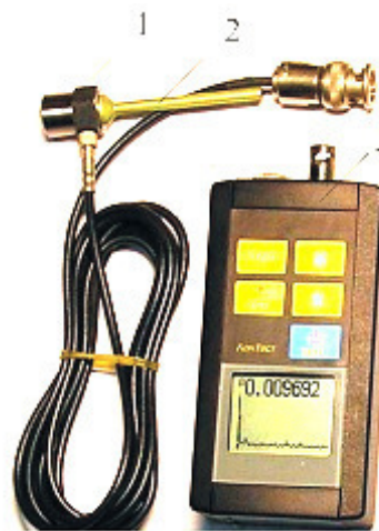
Figure 1 – Device for measuring vibration parameters «Vibrometer 107V»:
