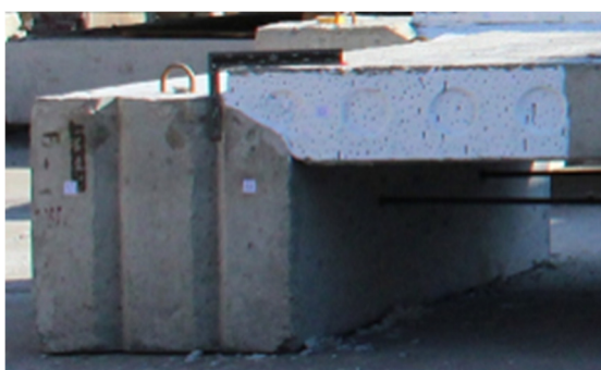
Figure 4 – Supporting blocks for testing of PMC series plates
