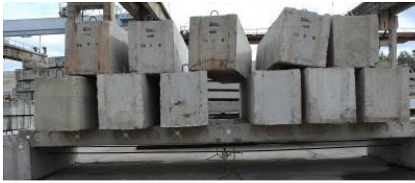
Figure 7 – Experimental sample of inter-column slab with pre-stressed working fittings during in-test
