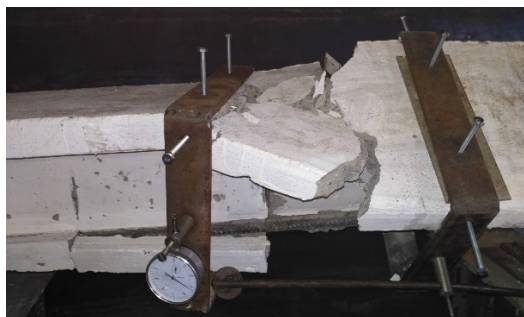
Figure 8 – Premature destruction of the beam as a result of puncturing the longitudinal reinforcement
